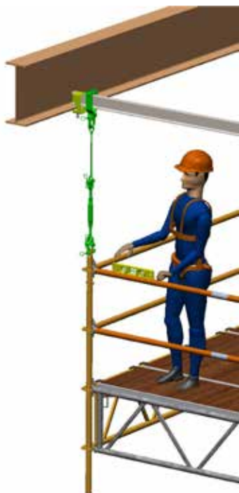
Fig. 5.14: Water levelling of the first completed bay by turning the turnbuckle before continuing with adjacent bays.
