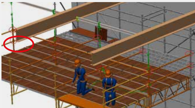
Fig.10.3: Safe tie-off points (red circles) at rosettes of suspended standards which are already mounted in a stabilized scaffold bay.
