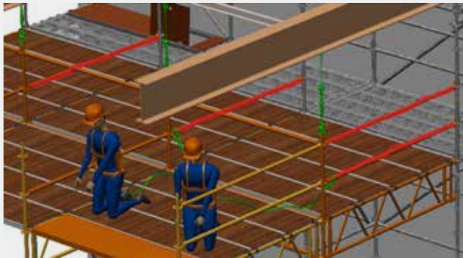
Fig.10.2: Safe tie-off points at ledgers (red lines) which are already mounted in a stabilized scaffold bay.
