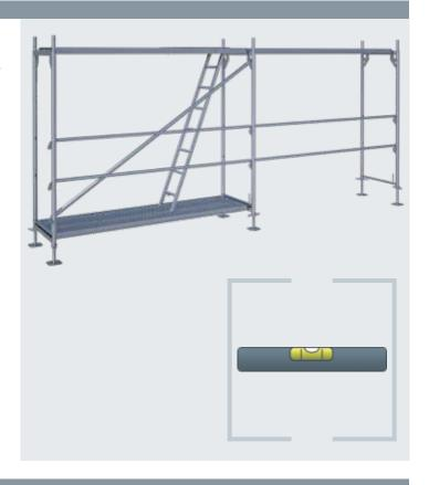
The assembly of the second level begins with the insertion of the vertical frames onto the frames of the first level. This thereby secures the lower decks on the first level.
