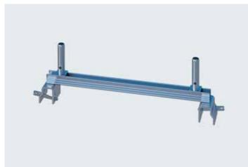
Attached to lattice girders or tubes and decked with FRAMESCAFF planks. For fitting additional scaffolding in modular bay dimensions in the case of bridging applications. Allows stepless decked levels in birdcage scaffolds. Comes with connecting pieces for guardrail supports.
