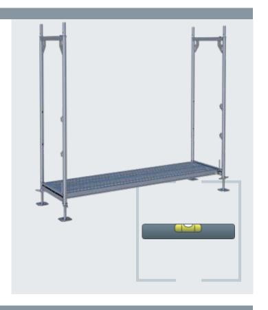
Diagonals and guardrails are fitted to the vertical frames. The frames are then aligned so as to be absolutely perpendicular and fixed there through the attachment of the diagonals. Decks provide the standing area for the next level. The first scaffold bay has now been established.
